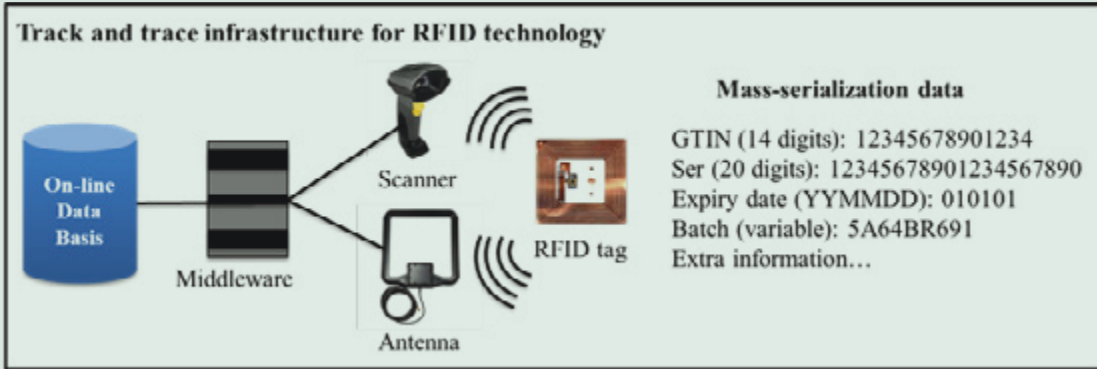
FIGURE 1. Track and trace system based on RFID technology
