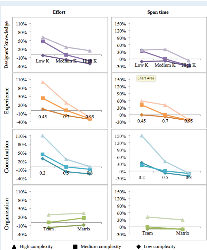
FIGURE 3. The effect of different factors on effort and span time under different levels of product complexity. Effort and span time are y-axis results, and knowledge, experience, coordination and organization are x-axis variables.
