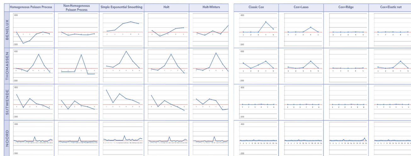
FIG 6. ANALYSIS OF EIGHT PROGNOSTIC METHODS FOR PREDICTIVE MAINTENANCE OF TUNNELS. THE Y-AXIS REPRESENTS THE DIFFERENCE BETWEEN THE REAL VALUE AND THE PREDICTION. THE PHM METHODS OF COLUMNS 6 TO 9 PERFORM BEST (NEDELICHEVA 2019).
